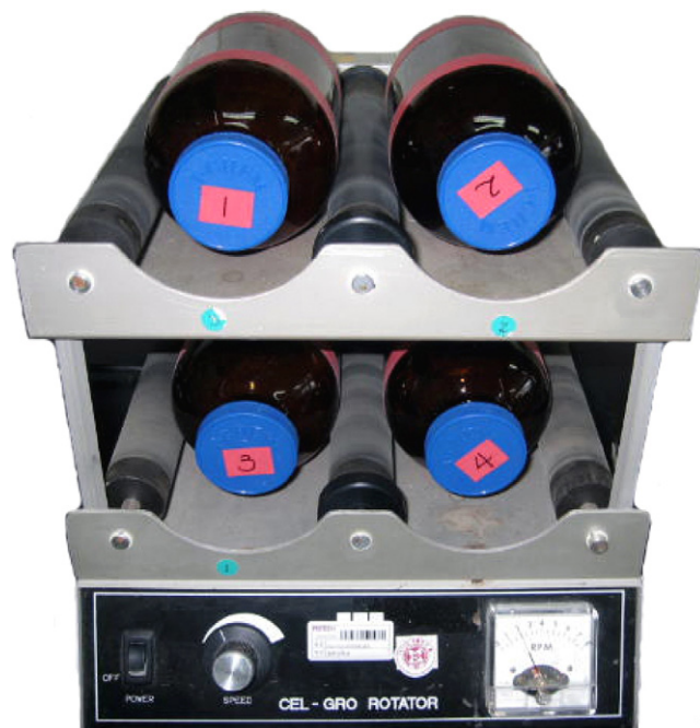
Fig. 1. Roller-bottles system used for ex situ soil remediation experiment in this study.
